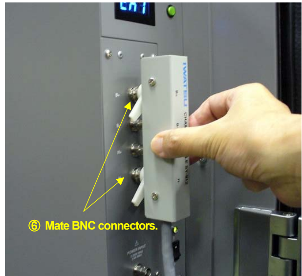
Fig.2-9 Connection of chamber cable
