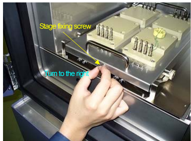
Fig.3-6 Installation of sample stage
