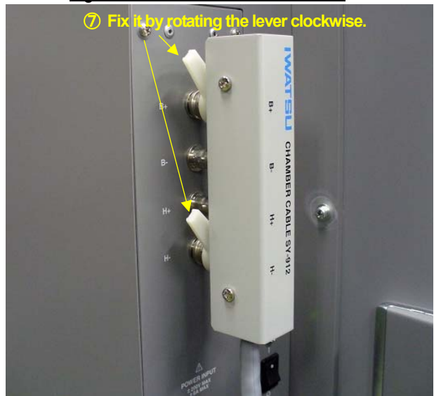
Fig.2-10 Connection of chamber cable
