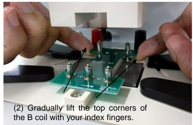
Fig. 4-11 Detaching a B coil
