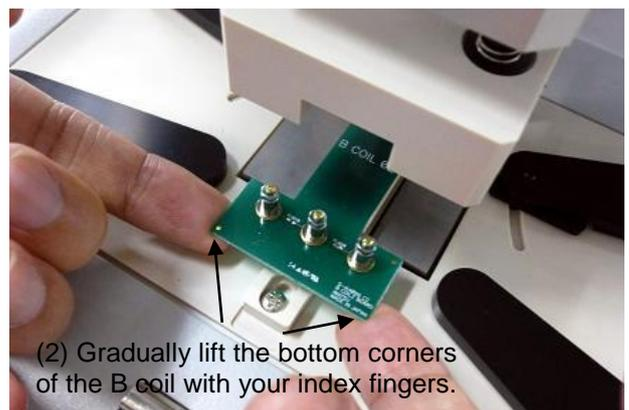
Fig. 4-12 Detaching a B coil
