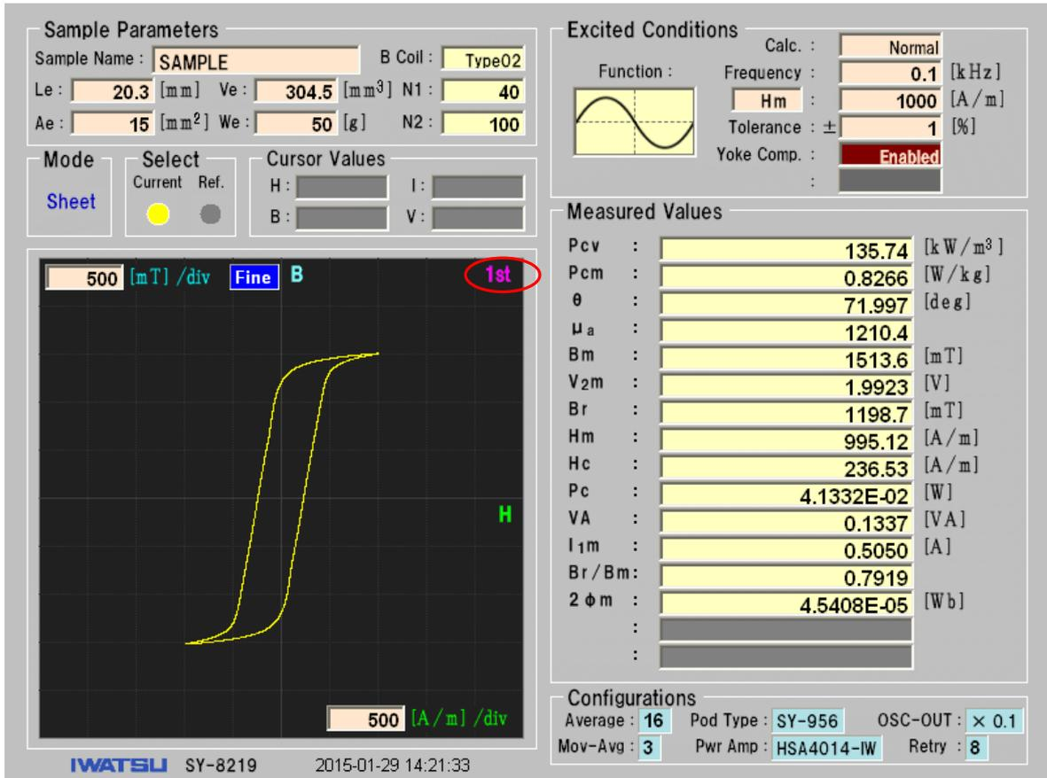
Fig. 4-19 1st Measurement Screen
