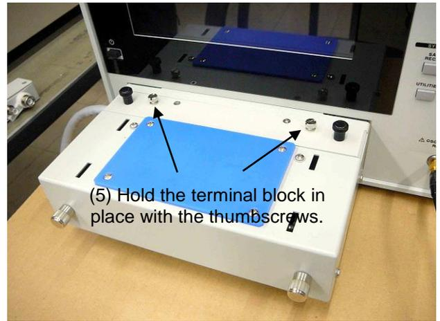
Fig. 4-7 Securing the SY-957 terminal block
