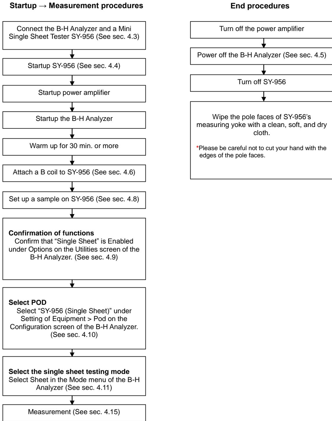
Fig. 4-1 Flow before measurement
