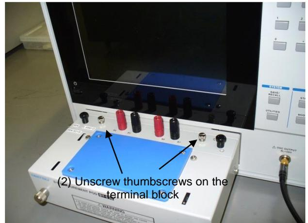
Fig. 4-3 Removing the measuring terminal block
