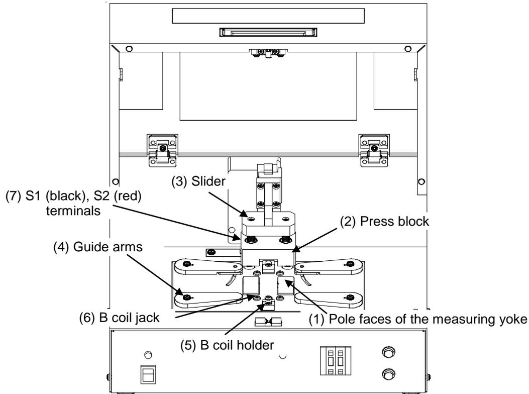
Fig. 3-2 Fixture of the SY-956
