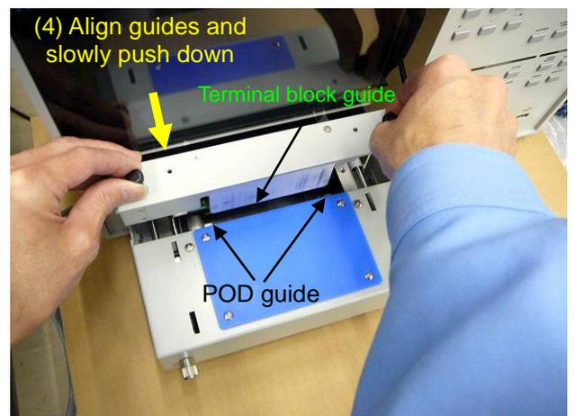
Fig. 4-6 Inserting the SY-957 terminal block
