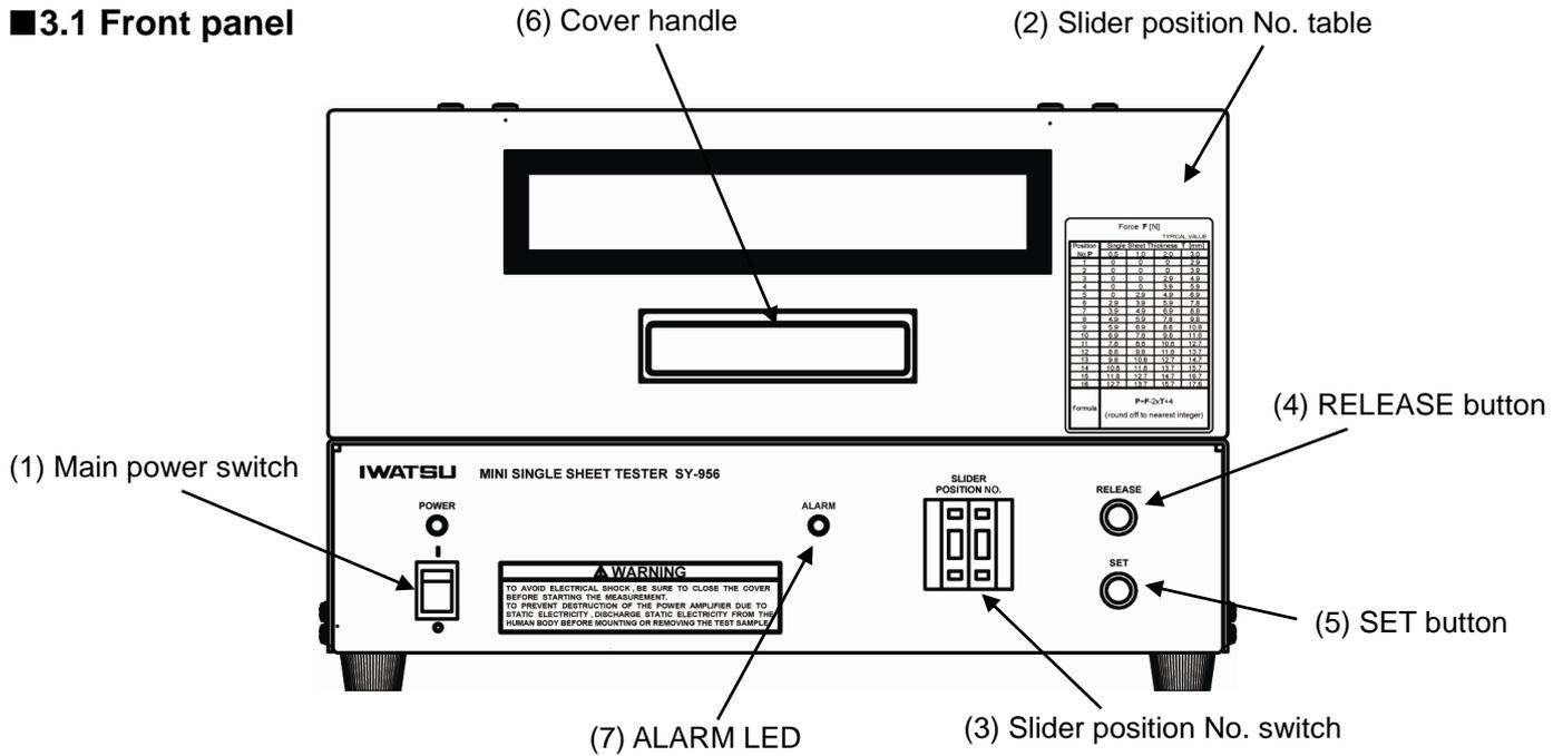
Fig. 3-1 Front Panel of SY-956
